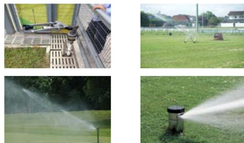
Fig. 3. Types of irrigation systems used in the sports turf industry. From left to right: canon type, self-travelling type, static type and pop-up type. Only automatic pop-up irrigation systems are considered appropriate for pitches used to host UEFA matches.
