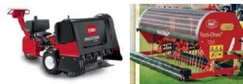
Fig. 21. Shallow aerator (left) and deep aerator (right).
